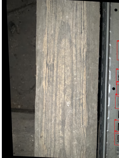
Figure 64: False detection of wood knots within the dataset Det-dominik-v3
