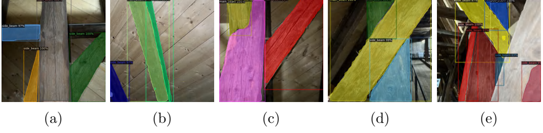
Figure 50: Images tested on test set of augmented Segdominik-v1 using model from M101_Test_5 with 13913 training iterations
