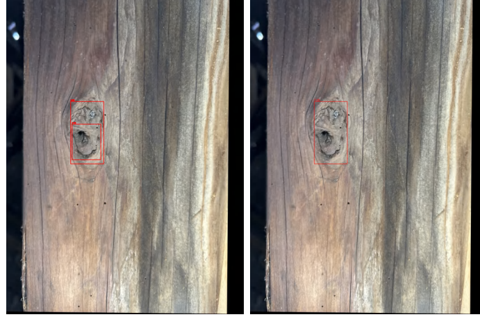
(a) Detection with bounding box overlapping (b) Detection after NMS refined
