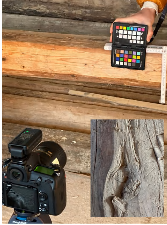
Figure 16: Perform color calibration prior to capture to standardize color accuracy
