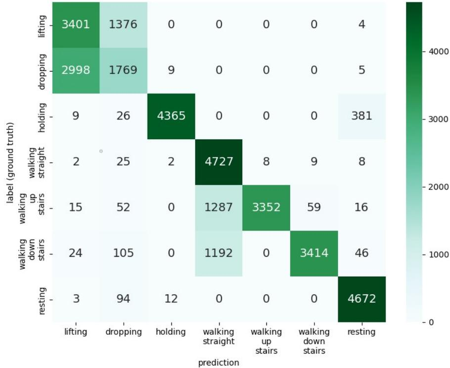
Figure 17: Confusion Matrix of the DeepFFNet Model on test data
