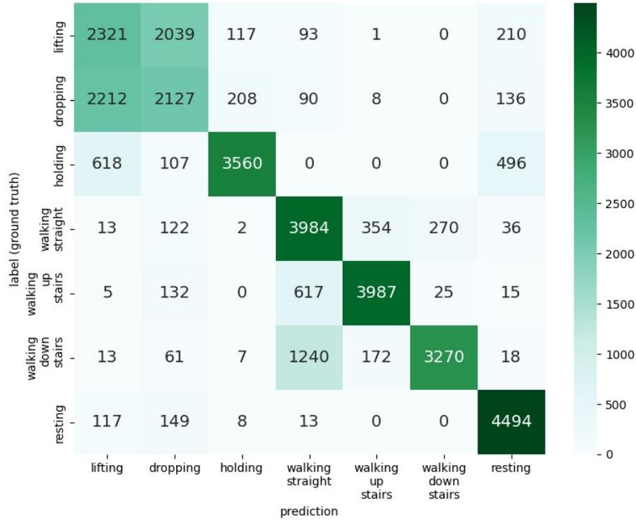
Figure 19: Confusion Matrix of the LSTMNet Model on test data
